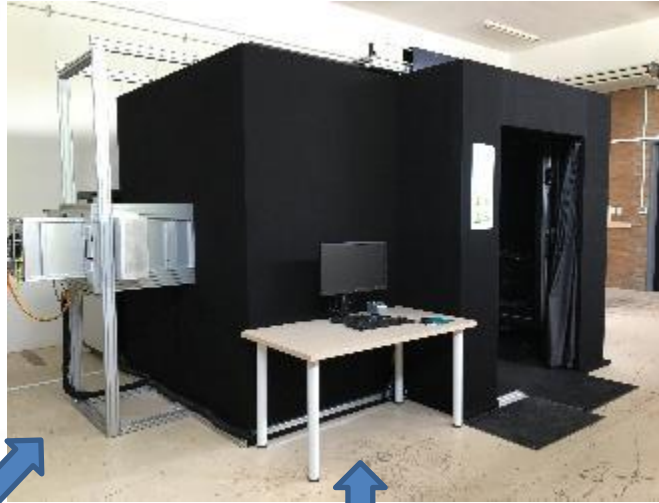
Sun simulator with temperature chamber
