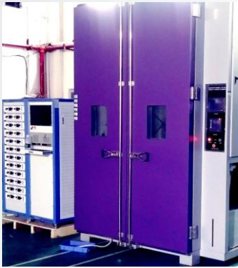
Thermal Cycling and Humidity Freeze with Power Supply Rack
